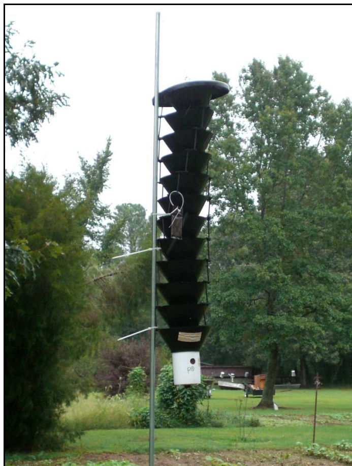
Figure 3: Lindgren funnel trap with lure packet, deployed near a TCD confirmed walnut tree in the Richmond, Virginia area. The lure packet can be seen attached to the outside of the trap about halfway down from the top.
